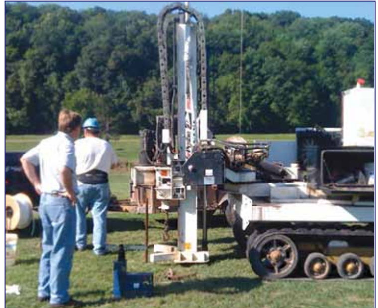
Ground water consultant geoprobng for salt contamination
